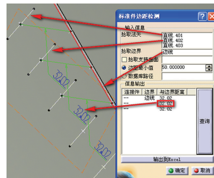
图9 手工输入最小边距查询结果 Fig.9 Querying results by manually entering the minimum margin
